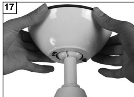
17 Raise the canopy up and align the two holes in the canopy with the two holes in the hanger bracket. Secure with two screws provided.
